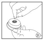
Insert the smaller cleaning wire into the single hole in the base of the filter.
